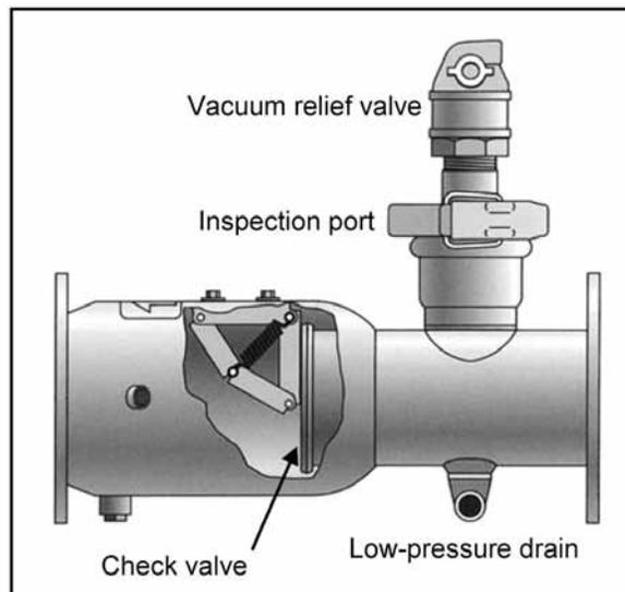
**Figure 2.** Irrigation mainline chemigation valve.
